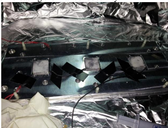
FIG 2.1 Heatsink baseplate with TEC mounted. The underside of the TEC has already been coated in thermal paste
