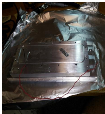
FIG 2.2 Assembled baseplate, including bottom plate of the main laser body
